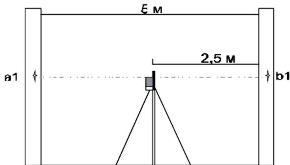
Set up the instrument 0,5-0,7m away from the wall and make, as described above, the same marks. If the difference  $\{a1-b2\}$  and  $\{b1-b2\}$  is less then the value of “accuracy” (see spesifications), there is no need in calibration.
